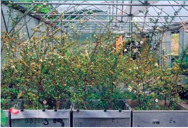
Trial containers for the root penetration test.
