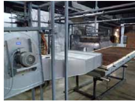
Testing equipment for test procedure 3: blower, radiant heater and a green roof build-up, initially without vegetation
