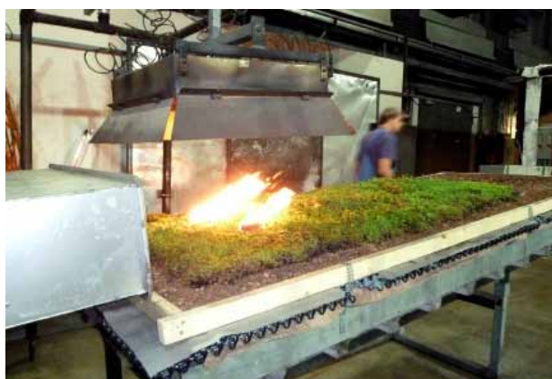
Testing equipment for test procedure 3 with a vegetation mat in place
