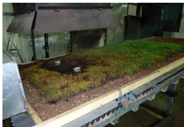
The 30 minute radiant heat led to the vegetation drying out across a diameter of about 80 cm
